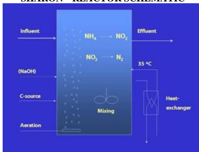
A characteristic feature of the reactor is that the biochemistry takes place without sludge retention that is the sludge retention time is equal to the liquid's hydraulic detention time;
