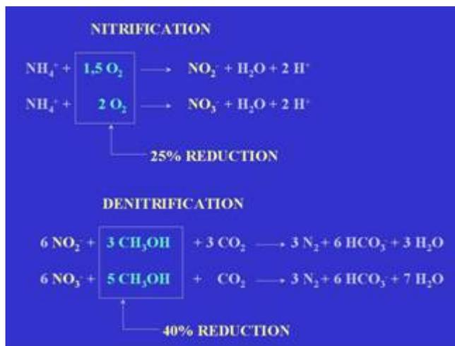
Since the oxidation of ammonia is taken only to nitrite and nitrite is reduced instead of being taken to nitrate and having the nitrate reduced there is a 25 % reduction in the oxygen requirements and a 40 % reduction in the carbon requirements.
