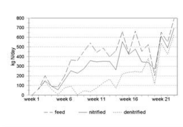
The average nitrogen load in the recycle stream was 520 kg N/ day. The feed to the reactor was not constant, but depended upon the amount of the plant's processed biosolids. The flow variation was between 0 and 980 m<sup>3</sup>/day. The recycle stream's ammonia concentration was on average 1230 mg N/l with a maximum of 1530 mg N/l, higher than the design value of 1000 mg N/l
