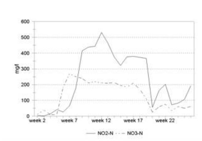
The initial removal of total nitrogen was above 90%. A malfunction of the instrumentation and control for pH caused this efficiency to decrease to 10%. The pH had dropped to 6.5. After repair and an increase in methanol dosing the pH increased to 7.0. The removal efficiency then steadily increased back to 90%. A similar trend was observed for ammonia nitrogen although the ammonia removal never dropped below 60%. (See Figure 10. "WEEKLY AVERAGED REMOVAL EFFICIENCIES")
