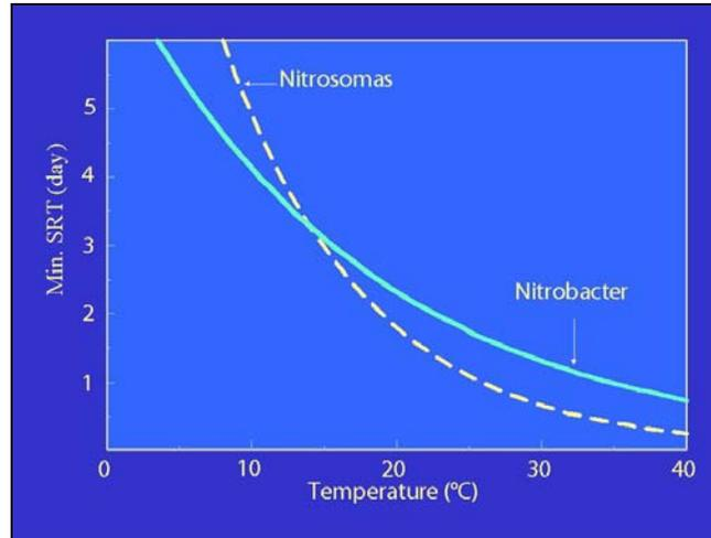
It is obvious from **FIGURE 3** that the reactor will operate best in the range from 25-40°C. The biological conversion of ammonia by this means with the influent at ammonia concentrations of about 1000 mgN/liter will cause a temperature rise of more than 10°C per gram of nitrogen removed per liter. Therefore heat production has to be considered in the process design.
