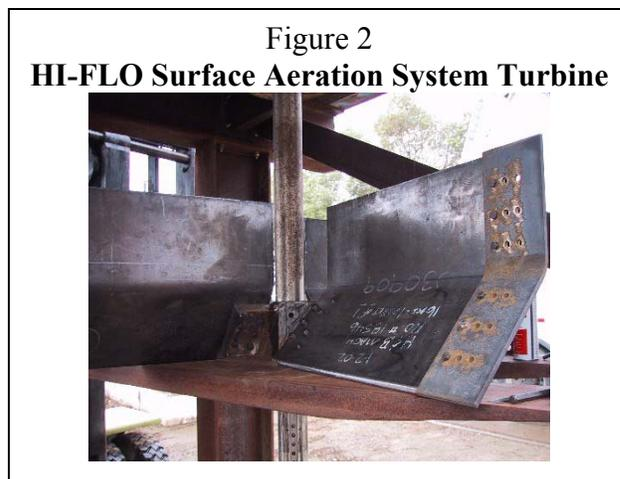
extender tabs that can be bolted onto the blade to increase the turbine's diameter. In general, sufficient "tips" were available for each size turbine to allow for increasing diameters in increments of approximately 4 inches, up to the maximum diameters shown in Table 1.
